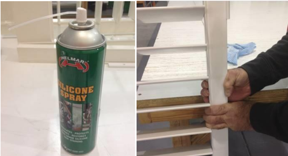
Can of Silicone Spray with nozzle. Step 2. Squeezing mech side of stile
